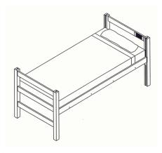
3. <u>Captain's Bed</u> Headboards right side up. Rails place on top pin location. A 3-drawer dresser can be positioned under the bed.
