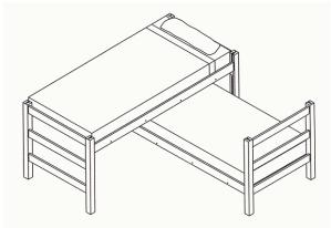
5. **Barrier Free Bed** Headboards are turned over. Rails use middle pin location. Mattress height is approx. 22".
