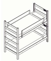
7. **Low Loft** Rail on back middle pin location for lower frame, rails on bottom pin location for top bed.
