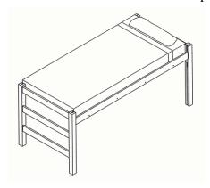
4. **L-Shaped Bed** Headboards right side up. Rails on bottom pin location for one bed, rails on top pin location for other bed. A 3-drawer dresser can fit beside lower bed.
