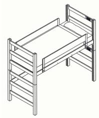
8. **<u>High Loft</u>** Rail of back middle pin location for lower frame, rails on middle pin location for the top bed. A desk and dresser can be positioned below the high loft.
