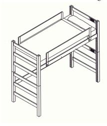
9. **<u>High Bunk Bed</u>** Rails on bottom pin location for the lower bed, rails on the middle pin location for the top bed.
